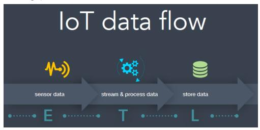
A typical IoT data flow involves a vast network of sensors publishing data periodically. That flux of information is then processed on the fly to extract patterns, trends, or execute predictions. Those end
